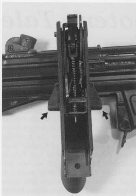
Top view of MP-5 three-shot lower. Ambidextrous selector levers can be seen on right and left sides (arrows).
