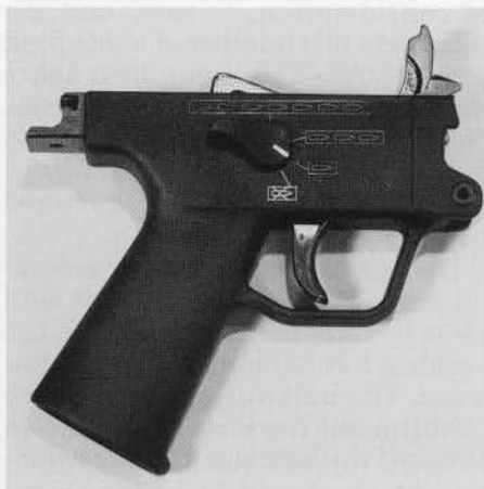
Three-shot mechanism and pistol grip assembly.
