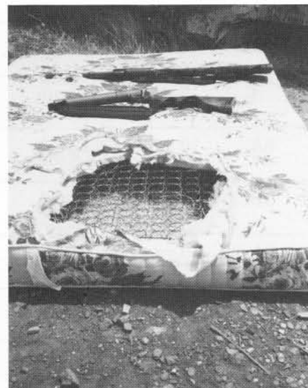
Wire spring coils inside of most mattresses help to rupture the caps of projectiles for close-in shots.
